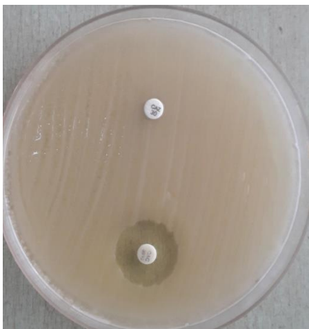
Fig. 1: Showing ESBL detection with combined disc diffusion method
