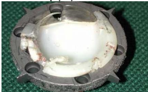
Plate 9: Shows severe wear and fracture of the polyethylene liner
