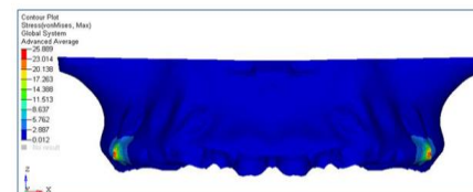
Figure 2b. Bone stresses with NiTi coil spring with miniscrew at 3 mm.
