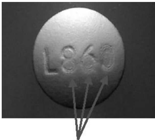
Fig.30: Erosion of the logo on the tablet
