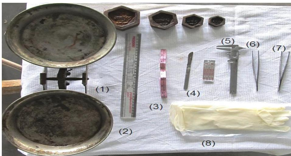
**Fig 22: Measuring instruments:** 1. Weighing machine with weights; 2. Measuring scale; 3. Measuring tape; 4. Scalpel with surgical blade; 5. Vernier calliper; 6. Forceps blunt; 7. Forceps toothed; 8. Gloves
